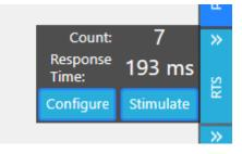
The response timer measures the patient's reaction time. The operator initiates the test by pressing the "Stimulate" button. This triggers a audio signal and the patient is supposed to respond by pressing the event button. The time between the stimuli and the button press is measured and indicated as the duration of the Reaction Time event. The Response timer is controlled from the Panel.
