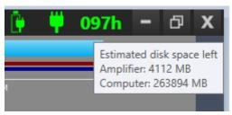
An indicator shows how much space is left on the amplifier memory card as hours and as MB on the tooltip. ER#17420.
