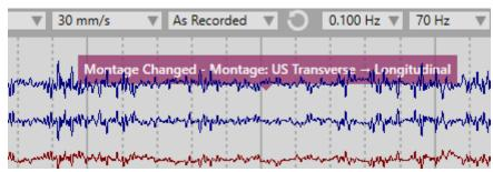
If setup or format is changed, an event is inserted with a description of the change. ER#17239.
