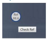
It is now possible to measure impedance on the reference electrode for Lifelines R40, T4 and T4A provided that that issue of the amplifier supports this function. This is done by pressing the "Check Ref" button during impedance test. Note that impedance on Ref cannot be tested at the same time as on the electrodes. ER#13238.
